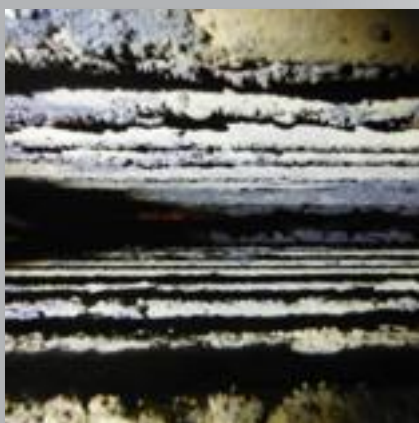
Deposits grow more rapidly. \Delta p increase. The deposits are corrosive, therefore, hard to remove and catalyse \text{SO}_2 to \text{SO}_3 .
